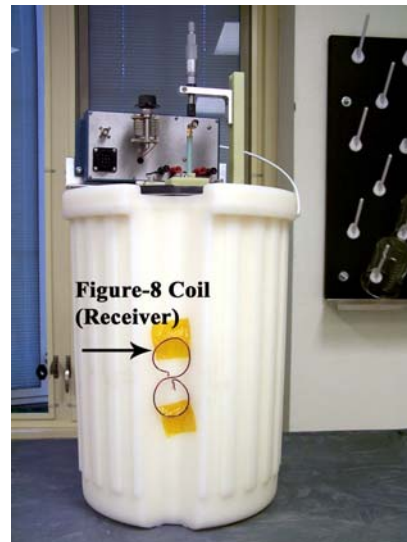
Figure 6: Outside of cryostat.
